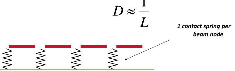
Large elements (10m and up to 30m) can be used on flat seabeds with limited dynamics
