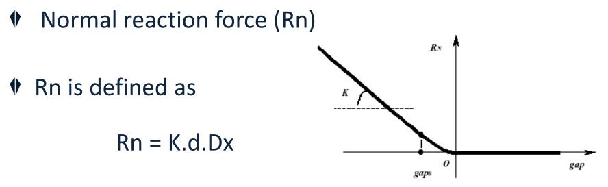
with Dx is the normal penetration, d the density of contact elements, and K the user-defined stiffness in N/m (a stiffness k = K/d is actually used)
