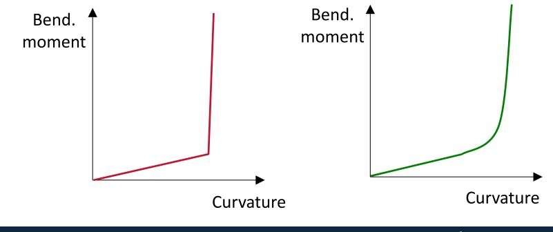
Use the Cable/Chain segment type when the bend stiffness is negligible instead of setting very low values in the Flexible segment type
