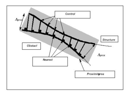
An iterative algorithm is used to find out the best position for contact elements during the simulation
